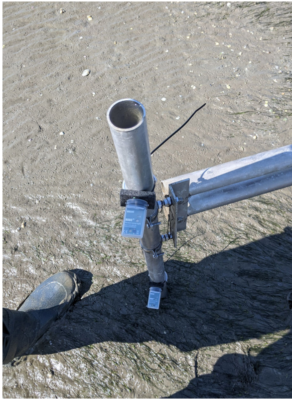
Fig. 6: Light-Loggers fitted on the pole of the multiparameter measurement probe rack
