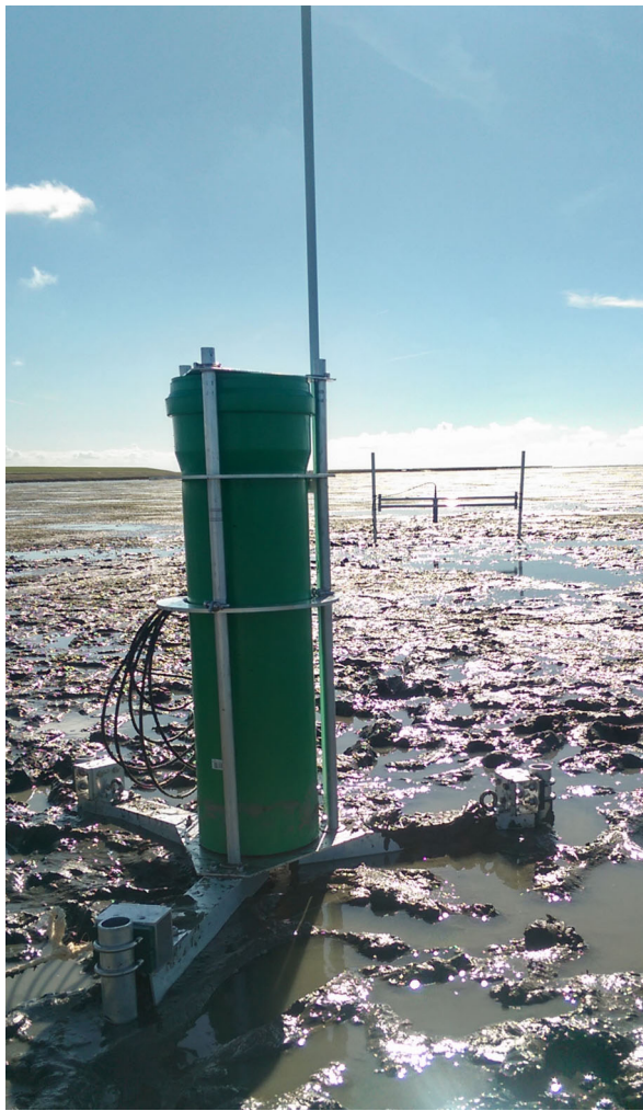
Fig. 2: Measurement station on the mainland shore site. In the foreground, the station's core contains the telemetry, power supply, and data-processing units; in the background, the probe collects the data, which is further processed in the central station.
