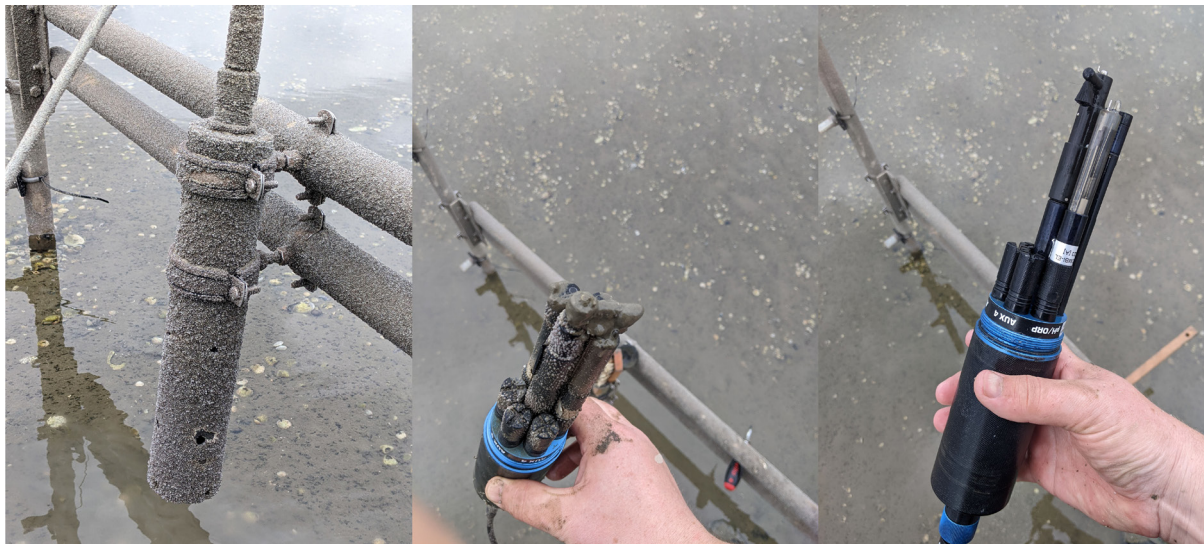
Fig. 4: Infestation with barnacles at the measurement station. Left: Heavy infestation on the probe. Center: Infestation on the sensors inside the protective casing. Right: Sensor after cleaning.
