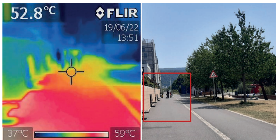
Fig. 5: Infrared image of the surface radiation temperature (LST) on a hot day in July 2022 on the 'Promenade' in Heidelberg's 'Bahnstadt' district. The area of the infrared image is indicated by the red rectangle. The path is paved with concrete and runs along a lawn and, on the other side, directly along the housing estate, separated by a wall of stamped concrete. The surface temperature visualisation also shows natural shading from trees, although this is minimal as the vegetation is relatively undeveloped due to new planting. There are a few benches, most of which are not shaded. The surface temperature has no direct effect on the air temperature as some of the energy is absorbed and later released through radiation. However, surface radiation also increases heat stress. The image therefore shows the significant overheating of the area at midday (indicated by the colour scale in degrees Celsius).
