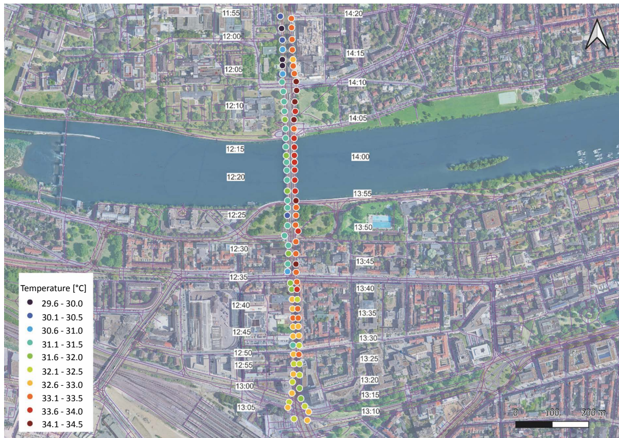
Fig. A2: Example of the on-site measurement data at Heidelberg, Bergheim along 'Mittermaierstraße'. Results show the overheating of the central city area and the dynamic temperature profile during midday on a heat day in July 2022.
