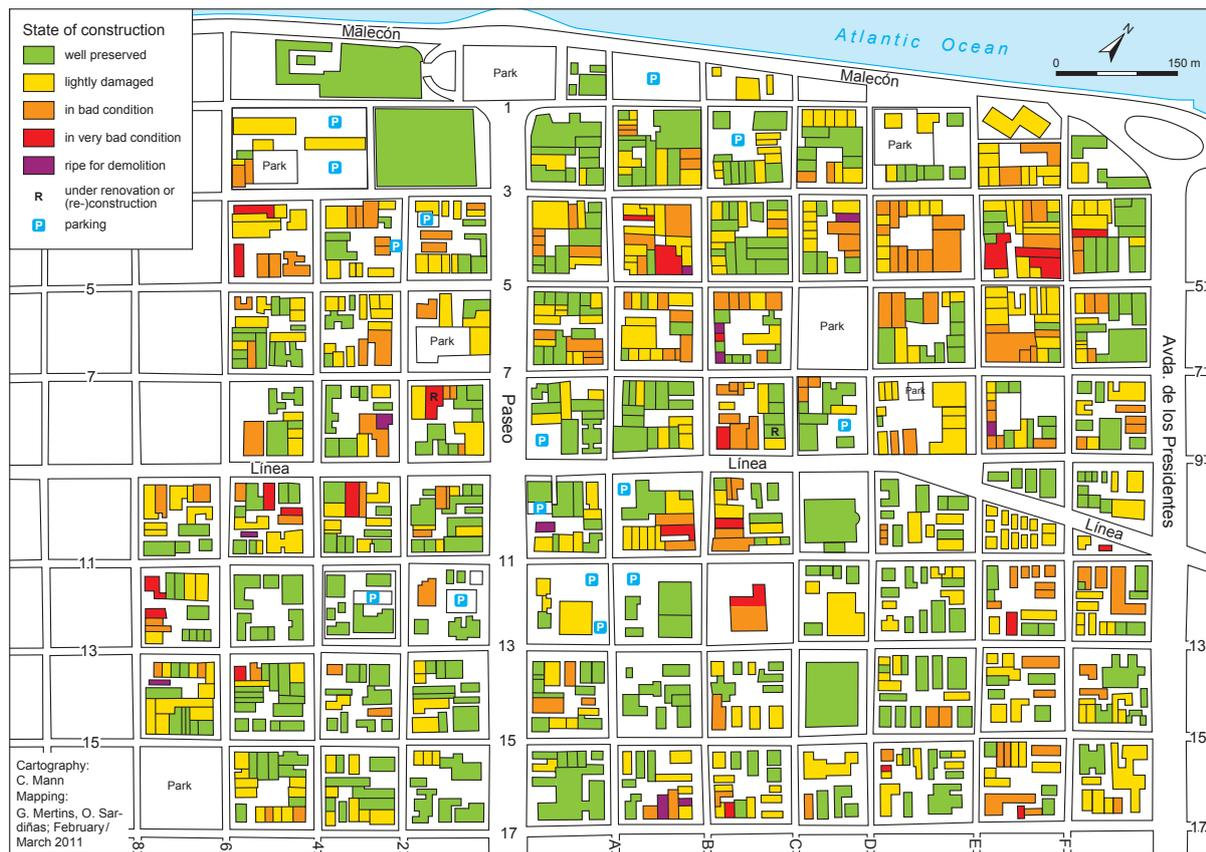
Fig. 3: El Vedado: state of building construction
