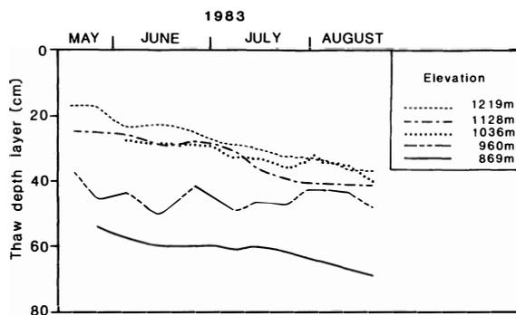
Fig. 1: Variations in mean thickness of the active layer at sites at different elevations along the vertical transect from May to August, 1983. Each data point is based on the mean of 10 measurements
